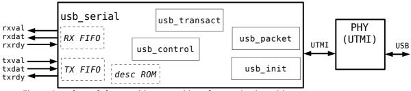
Figure 1: usb\_serial core with external interface and sub-entities
